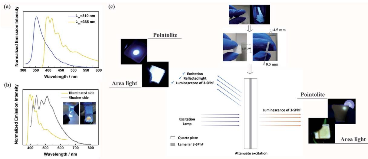
Fig. 6 (a) Normalized steady-state PL spectra of 3-SPhF at different excitation wavelengths; (b) PL spectra of illuminated and shadow sides for the 3-SPhF crystal powder ( $\lambda_{ex} = 365$  nm); (c) photographs and mechanism for different color emissions of lamellar compounds at illuminated and shadow sides.
