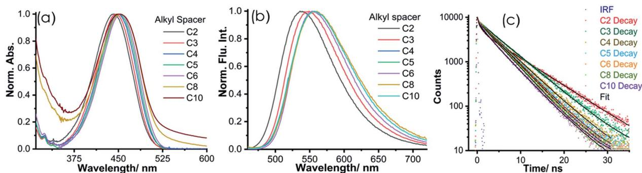
Fig. 3 Representation of photophysical properties: (a) absorption, (b) emission ( $\lambda_{\text{ex}} = 450$  nm), and (c) emission lifetime of the synthesized NIMCs in water (pH = 6.0), where the fluorescence decays were recorded using a 440 nm excitation LASER.
