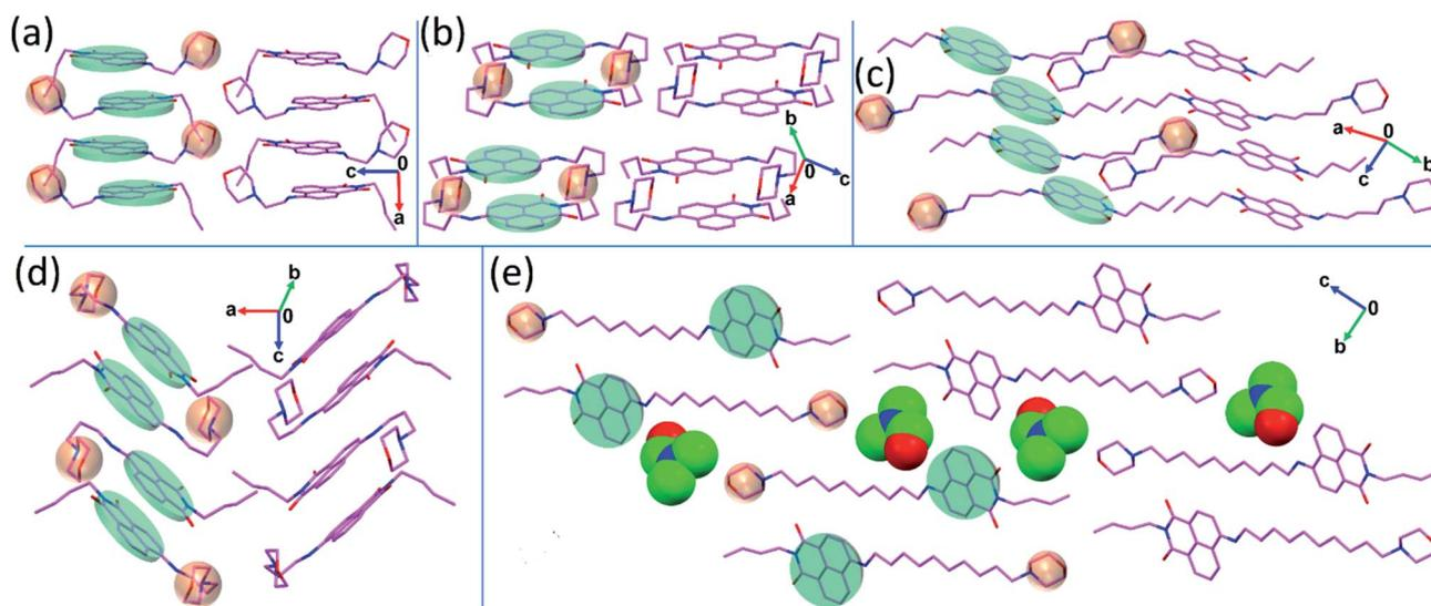
Fig. 1 Representation of the solid-state geometry of the synthesized **NIMCs**, (a) **NIMC2**, (b) **NIMC3**, (c) **NIMC5**, (d) **NIMC4** and (e) **NIMC10** obtained from the single-crystal X-ray diffraction. Crystal packing reveals that the molecules are stacked *via*  $\pi \cdots \pi$  interactions and the shorter alkyl spacers adopt a bent chain conformation, while a straight chain geometry is adopted by intermediate and longer alkyl spacers.
