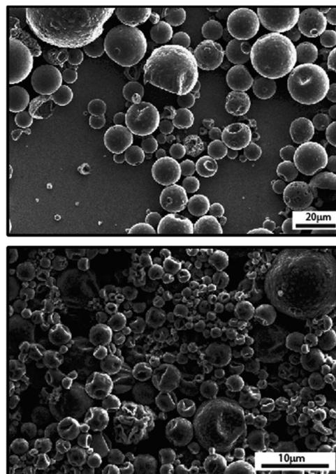
Fig. 4 SEM micrographs of [BMIM][PF<sub>6</sub>] in polyurea capsules prepared *via* emulsion polymerization in water (top) and in oil (bottom). [Reprinted from *React. Funct. Polym.*, Weiss, E.; Gertopski, D.; Gupta, M. K.; Abu-Reziq, R. Encapsulation of Ionic Liquid BMIm[PF<sub>6</sub>] within Polyurea Microspheres. 2015, 96, 32–38, with permission from Elsevier].<sup>42</sup>
