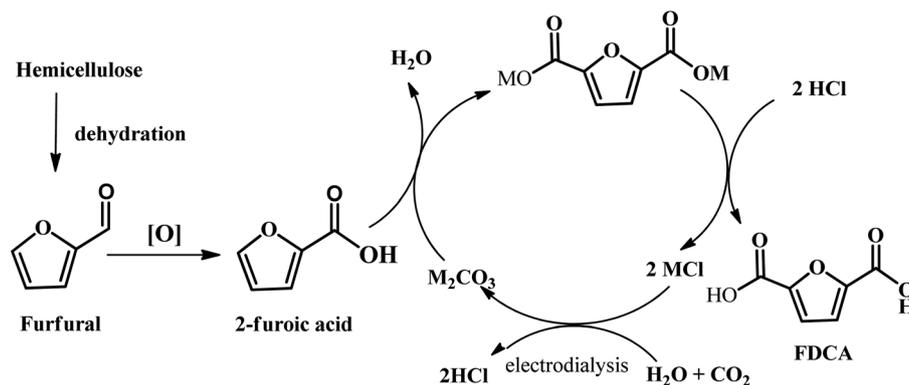
Fig. 8 Schematic illustration of the overall diagram for the production of FDCA from biomass through furfural using  $\text{CO}_3^{2-}$ -promoted C–H carboxylation. Recovery of the alkali cations is achieved by protonation of the FDCA salt and bipolar membrane electro dialysis of the resulting alkali chloride salt. Reprinted from ref. 67. Copyright 2016, The Royal Society of Chemistry.
