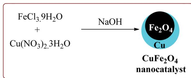
Scheme 43 Preparation of CuFe<sub>2</sub>O<sub>4</sub> nanocatalyst.
