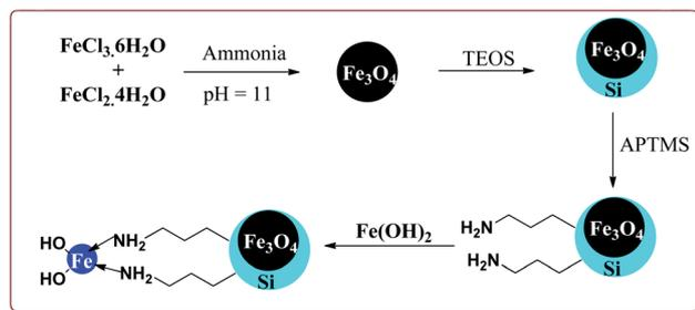
Scheme 36 Preparation of  $\text{Fe}_3\text{O}_4@\text{SiO}_2\text{-APTMS-Fe(OH)}_2$  nanocatalyst.
