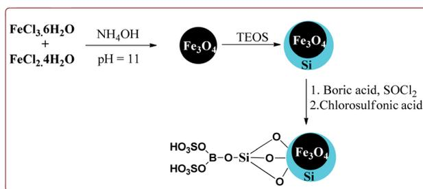
Scheme 38 Synthesis of sulfated boric acid-silica-coated magnetite nanoparticles.
