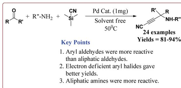
Scheme 29 Synthesis of  $\alpha$ -amino nitriles derivatives by using urea and urethane based four novel magnetic nanocatalysts.
