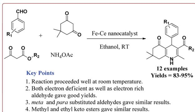
Scheme 41 Synthesis of 1,4-dihydropyridines catalyzed by Fe-Ce nanocatalyst.
