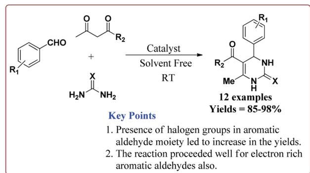
Scheme 37  $\text{Fe}_3\text{O}_4@\text{SiO}_2\text{-APTMS-Fe(OH)}_2$  catalyzed Biginelli reactions.
