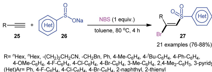
Scheme 12 Catalyst-free direct bromosulfonylation of terminal alkynes 25 with sodium arylsulfonates 26 employing NBS as the bromine source.
