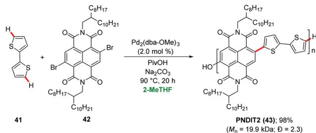
**Scheme 14** Palladium-catalyzed direct C–H arylation polymerization in 2-MeTHF.
