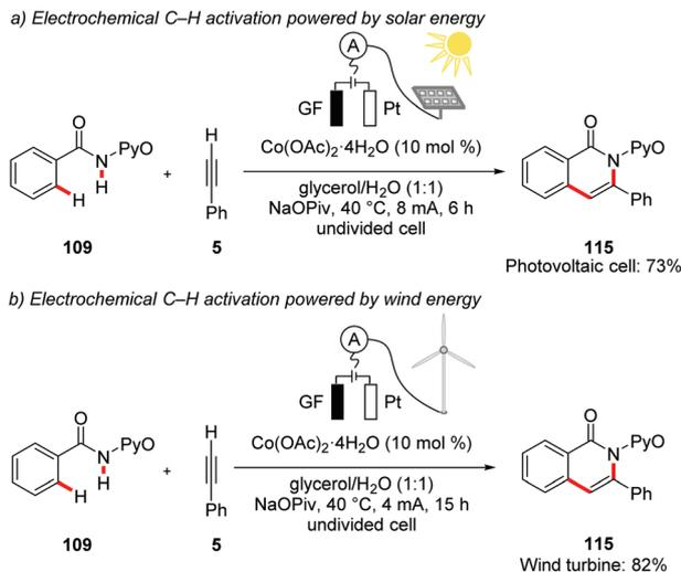
**Scheme 38** Electrochemical C–H activation powered by renewable electricity.
