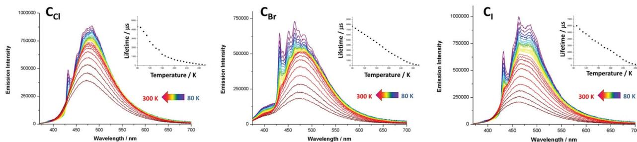
**Fig. 3** Temperature dependence (80 K to 300 K) of the solid-state emission spectra of metallacycles C<sub>Cl</sub>, C<sub>Br</sub> and C<sub>I</sub> upon excitation at 325 nm. ‡ Inset: plot of their emission decay lifetime against temperature (80 K to 300 K).
