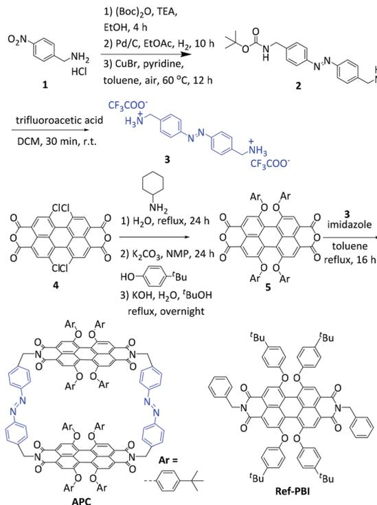
**Scheme 1** The synthetic route towards PBI cyclophane **APC**. In addition, the chemical structure of **Ref-PBI**<sup>27</sup> is shown, which is used as a reference compound.
