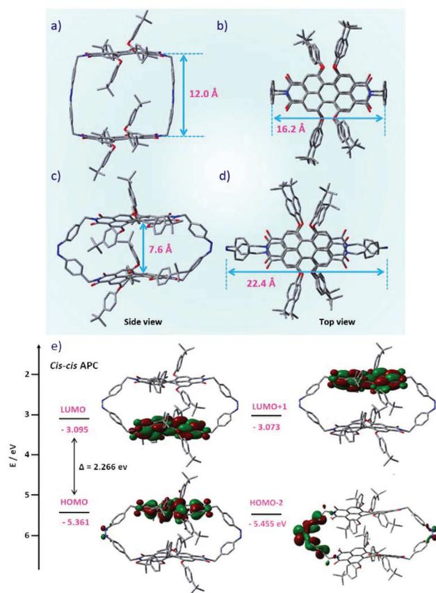
**Fig. 5** Density functional theory calculated structures of (a and b) *trans-trans* APC and (c and d) *cis-cis* APC. (e) Illustration of energy levels and molecular orbitals of *cis-cis* APC. Gaussian 09, B3LYP/6-31G (d,p) level. All hydrogen atoms are omitted for clarity.
