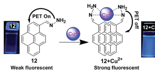
Fig. 13 Schematic representation of \text{Cu}^{2+} sensing by fluorosensor 12 and emission photograph of 12 and 12 + \text{Cu}^{2+} under UV radiation. Reproduced from ref. 78, with permission from the Royal Society of Chemistry.
