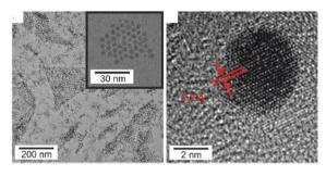
Fig. 16 TEM images of  $Cu_3N$  NCs synthesized by sol-gel chemistry according to ref. 126. Reproduced from ref. 126 with permission from the Royal Society of Chemistry.
