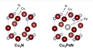
Fig. 11 Crystal structure of  $Cu_3N$  and the doped  $Cu_3PdN$ . The copper is represented in dark red, the palladium in grey and the nitrogen atom in cyan. Structures plotted using VESTA.<sup>48</sup> Cif file obtained from ref. 111 and 112.
