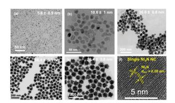
Fig. 10 TEM images of the different Ni<sub>3</sub>N NCs obtained. (a)  $5.6\pm0.9$  nm, (b)  $10.6\pm1.0$  nm, (c)  $36.6\pm0.8$  nm, (d)  $56.4\pm6.5$  nm, and (e)  $76.4\pm3.8$  nm. (f) High resolution transmission electron microscopy (HRTEM) imageof a Ni<sub>3</sub>N nanocrystal with a size of  $56.4\pm6.5$  nm. Reprinted with permission from ref. 97. Copyright 2021 American Chemical Society.
