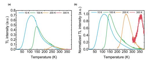
Fig. 6 (a) TL curves of an m-MTDATA/PPT film. The sample was photoexcited at the starting temperature (10 K, 100 K, 200 K, and 300 K) for 300 s. After 1 h, the sample temperature was increased at 5 K min<sup>-1</sup>. (b) Normalized TL curves.
