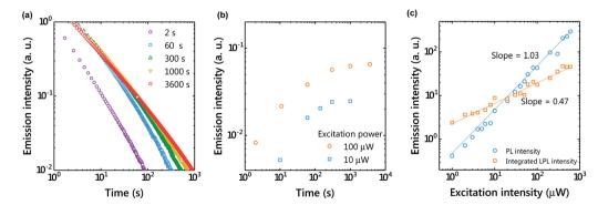
Fig. 3 (a) Emission decay profiles showing the dependence of LPL on the excitation time (1 molar ratio of the donor; excitation power, 100 μW; temperature, 300 K), (b) Excitation-time dependence of the emission intensity 100 s after photoexcitation, (c) Excitation-power dependence of the emission intensity under photoexcitation (PL) and integrated LPL intensity. The LPL intensity was integrated from 100 s to 10 000 s after photoexcitation. The solid lines show linear fitting.
