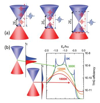
Fig. 13 (a) THG in graphene is enhanced at specific values of  $E_{\rm F}$  corresponding to one-, two- and three-photon transitions within the Dirac cone. (b) The increase of  $T_{\rm e}$  affects the nonlinear conversion efficiency by broadening the electron distribution. The graph shows the THG efficiency, defined as  $I_{3\omega}/I_{\omega}$ , for  $\hbar\omega$  = 500 meV and a peak power density of ~230 MW cm<sup>-2</sup>.
