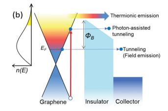
Fig. 17 (a) Schematic of interlayer transport and intralayer thermalization of photoexcited carriers in a g/hBN/g heterostructure. (b) Band diagram of a graphene heterostructure illustrating various interlayer transport mechanisms. The yellow shaded area in the hot-carrier distribution n(E) represents the carriers with an energy larger than the barrier  $\Phi$  that can generate thermionic emission. Panel (a) is reproduced with permission from ref. 216 (Copyright 2016 Springer Nature).
