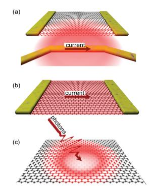
Fig. 2 Schematic illustrations of (a) thermal excitation, (b) electrical excitation, and (c) optical excitation.
