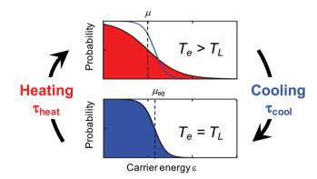
Fig. 1 Illustration of heating-cooling dynamics of graphene carriers, where in the hot state the carrier distribution is characterized by an increased carrier temperature  $T_{\rm e}$  that is larger than the lattice temperature  $T_{\perp}$  and a "hot" chemical potential  $\mu$  that is smaller than the equilibrium chemical potential  $\mu_{eq}$
