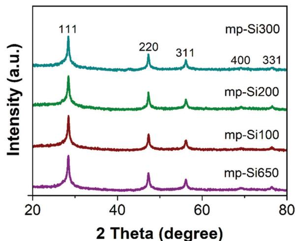
Fig. 1 Powder XRD patterns of mp-Si NPs prepared using a single heating step magnesiothermic reduction process at  $650^\circ\text{C}$  for 3 h (mp-Si650) and two heating steps with the second annealing temperature of  $100^\circ\text{C}$  (mp-Si100),  $200^\circ\text{C}$  (mp-Si200), and  $300^\circ\text{C}$  (mp-Si300).
