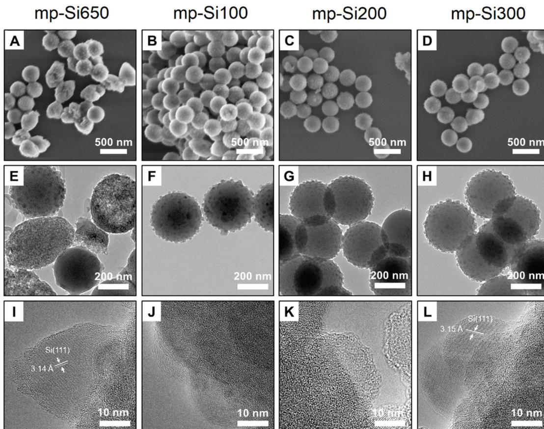
**Fig. 2** (A–D) SEM, (E–H) TEM, and (I–L) HRTEM images of mp-Si NPs prepared under different magnesiothermic reduction conditions. mp-Si650 was prepared using the single step heating at 650 °C for 3 h. mp-Si100, mp-Si200, and mp-Si300 were prepared using the two step heating method with the second annealing temperature of 100, 200, and 300 °C, respectively.
