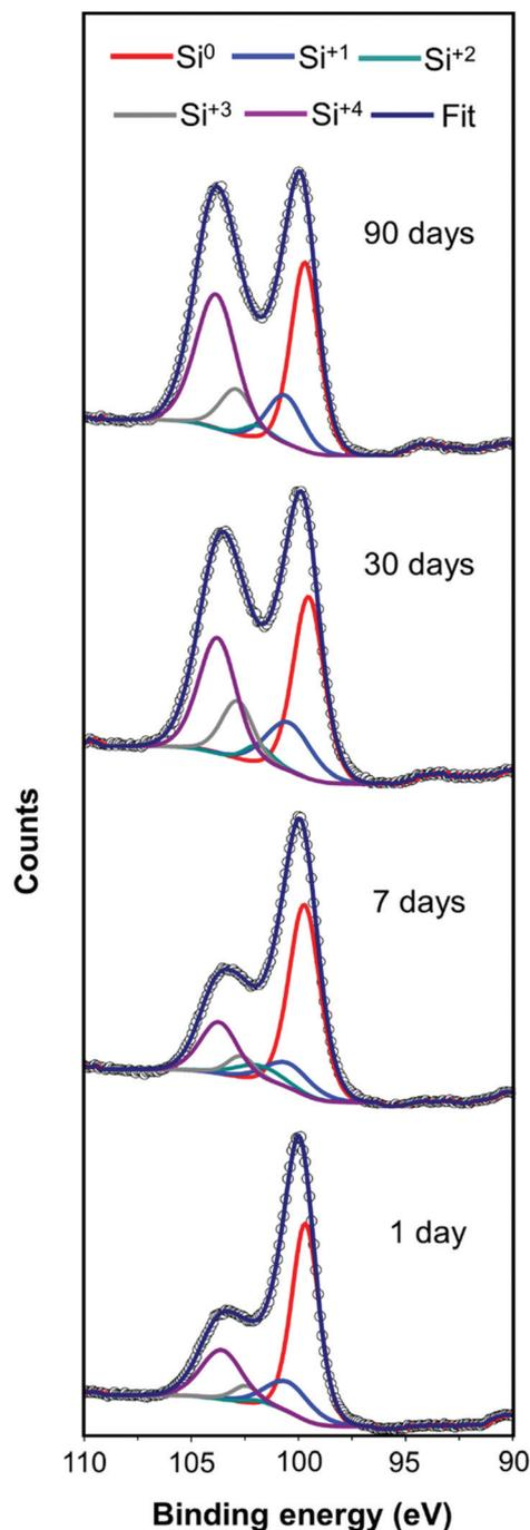
**Fig. 5** High resolution XP spectra of the Si 2p region of mp-Si300 NPs at different times after the synthesis and storage under ambient conditions. For clarity, only 2p<sub>3/2</sub> peaks of different oxidation states are shown.
