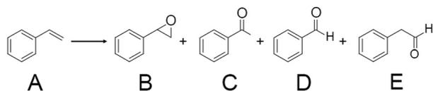
**Scheme 4** Styrene oxidation using metal NC catalysts. In this reaction, typically, TBHP is used as an oxidant because it is known to be more effective than O<sub>2</sub> for alkene oxidations.<sup>219</sup> The reaction was conducted in toluene or acetonitrile in the literature.<sup>219–224</sup> A = styrene, B = styrene oxide, C = acetophenone, D = benzaldehyde, E = 3-phenylpropionic acid. In ref. 219, by-products such as benzoic acid and benzyl alcohol are also produced.
