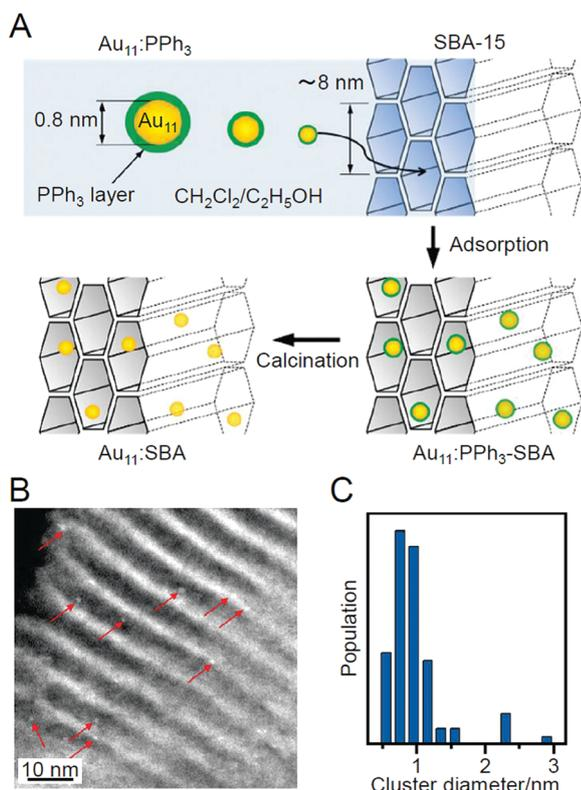
Fig. 3 (A) Synthesis procedure of sub-nanometer-sized Au NCs within SBA-15 using PPh<sub>3</sub>-protected Au<sub>11</sub> NCs as a precursor. (B) Representative HAADF-STEM image and (C) size distribution of Au NCs prepared by adsorption method. Reproduced with permission from ref. 183. Copyright 2009 American Chemical Society.
