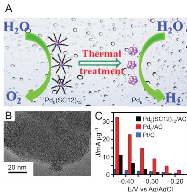
Fig. 30 (A) Schematic of difference in electrochemical reaction before and after thermal treatment of Pd<sub>6</sub>(SC12)<sub>12</sub>/AC (B) HR-TEM images of Pd<sub>6</sub>/AC. (C) Comparison of the current densities of the HER on the samples at different potentials. Reproduced with permission from ref. 246. Copyright 2017 Royal Society of Chemistry.
