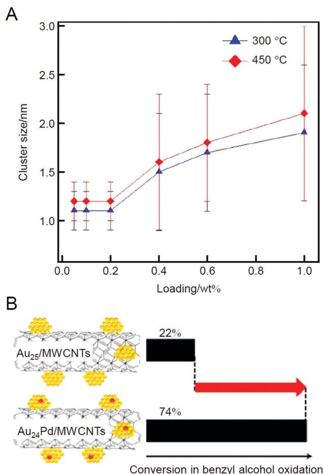
Fig. 4 (A) Dependence of the loading amounts of Au<sub>25</sub> NCs on the Au particle size in Au<sub>25</sub>/MWCNTs. The error bars indicate the size distribution determined by TEM. (B) Catalytic performances of Au<sub>25</sub>/MWCNTs and Au<sub>24</sub>Pd/MWCNTs for benzyl alcohol oxidation. Reproduced with permission from ref. 209. Copyright 2012 American Chemical Society.
