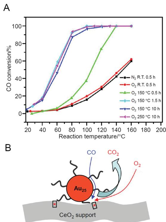
**Fig. 16** (A) Reaction temperature dependence of CO conversion over Au<sub>25</sub>(PET)<sub>18</sub>/CeO<sub>2</sub> catalyst after different pre-treatments. Gas hourly space velocity (GHSV) = 7500 mL g<sup>-1</sup> h<sup>-1</sup>. (B) Proposed model for CO oxidation at the perimeter sites of Au<sub>25</sub>(PET)<sub>18</sub>/CeO<sub>2</sub> catalyst. Reproduced with permission from ref. 226. Copyright 2012 American Chemical Society.
