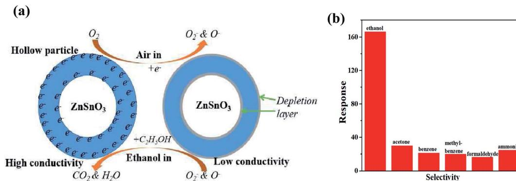
Fig. 17 (a) Ethanol sensing mechanism of  $\text{ZnSnO}_3$  hollow particles. (b) Sensing response ( $R_3/R_0$ ) of  $\text{CNT@ZnSnO}_3$  exposed to different types of gases, i.e. ethanol, acetone, benzene, methyl-1-benzene, formaldehyde and ammonia (from left to right)<sup>216</sup> (reprinted from ref. 216, Copyright (2020), with permission from Elsevier).
