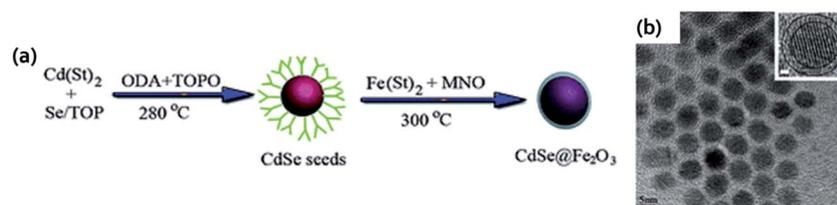
Fig. 8 (a) Scheme for the synthesis of CdSe@Fe<sub>2</sub>O<sub>3</sub> core-shell nanoparticles and (b) HRTEM image of the MFNPs. Reproduced from ref. 107 with permission from Royal Society of Chemistry, copyright 2011.
