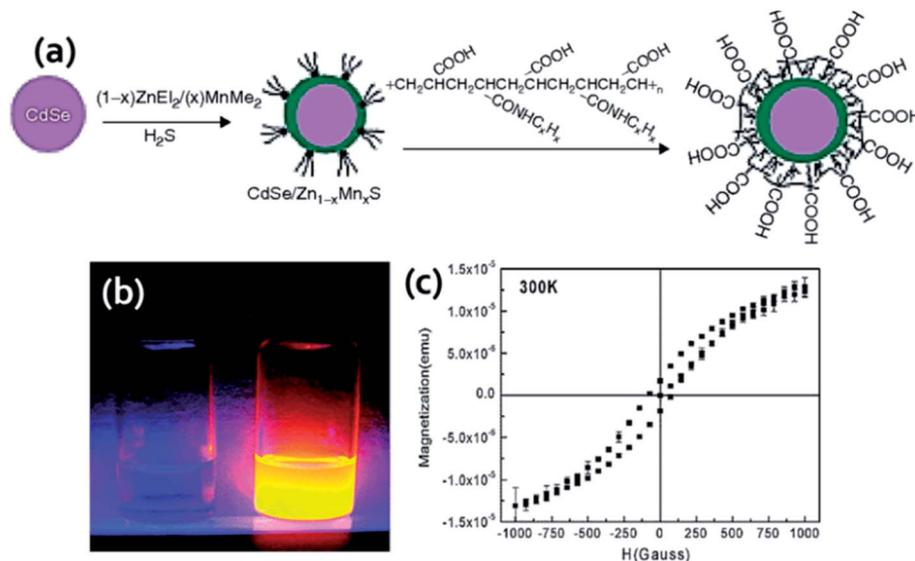
Fig. 2 (a) Synthesis procedure for the fabrication of water soluble core/shell CdSe/Zn<sub>1-x</sub>Mn<sub>x</sub>S. Reproduced from ref. 65 with permission from American Chemical Society, copyright 2007. (b) Fluorescence of yellow-emitting QDs (right) and DI water (left) under 366 nm UV source and (c) magnetization curve for QDs. Reproduced from ref. 70 with permission from American Chemical Society, copyright 2005.
