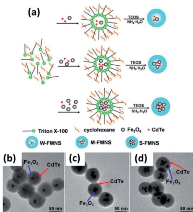
Fig. 5 (a) Schematic of the preparation of  $(\text{CdTe}/\text{Fe}_3\text{O}_4)@-\text{SiO}_2$  FMNS with various magnetic potentials *via* reverse microemulsion method. TEM images of  $(\text{CdTe}/\text{Fe}_3\text{O}_4)@-\text{SiO}_2$  FMNS: (b) W-FMNS, (c) M-FMNS, and (d) S-FMNS. Reproduced from ref. 99 with permission from American Chemical Society, copyright 2014.
