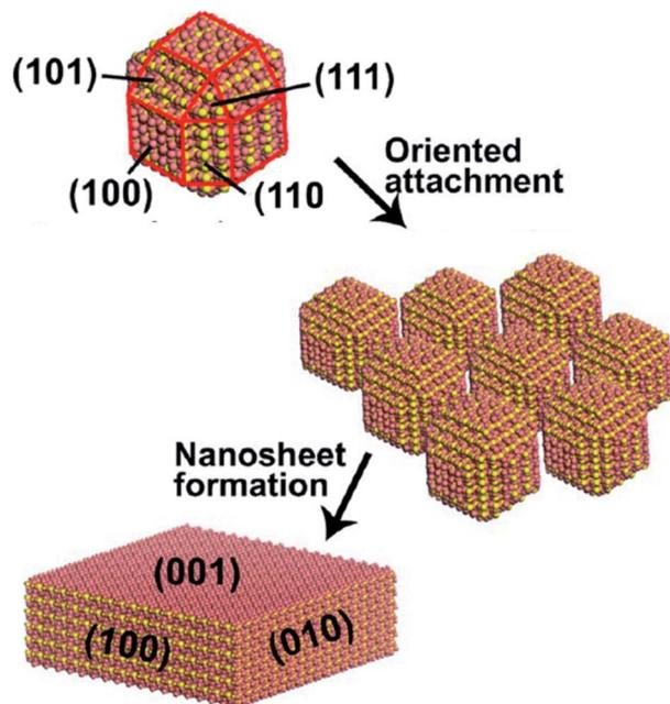
Fig. 5 Schematic of  $\text{WO}_3$  formation from smaller nanocrystals produced through solid-liquid phase arc discharge. Reprinted with permission from ref. 24, copyright 2012, American Chemical Society.
