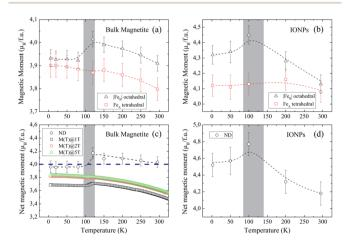
Fig. 5 Thermal variation of the Fe<sub>A, B</sub> magnetic moment for (a) bulk magnetite and (b) IONP samples. Thermal evolution of the net magnetic moment per formula unit (f.u.) for (c) bulk magnetite and (d) IONPs. The blue dashed line corresponds to the theoretical net moment value for stoichiometric magnetite. Dashed lines are guides to the eye.
