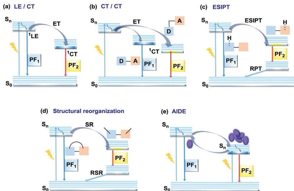
Fig. 2 Jablonski diagrams, presenting an overview of the processes in (a) LE/CT, (b) CT/CT, (c) ESIPT, (d) structural reorganization and (e) AIDE types of prompt DE. ET – electron transfer; RPT – reverse proton transfer; SR – structural reorganization; RSR – reverse structural reorganization; AIDE – aggregation induced dual emission.
