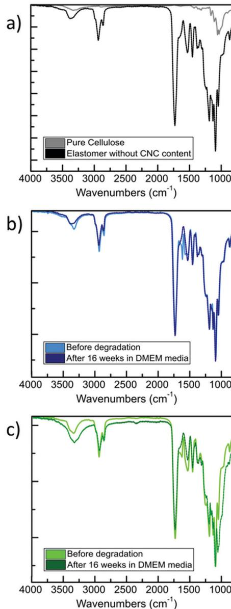
Fig. 4 FT-IR spectra for: (a) pure elastomer and neat CNCs; (b) 6A-PCL-LCE matrix containing 5 wt% CNC before and after 16 weeks *in vitro* degradation; (c) 6A-PCL-LCE matrix containing 40 wt% CNC before and after 16 weeks *in vitro* degradation.
