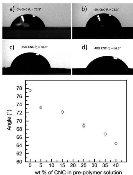
Fig. 9 Contact angle images for composites containing (a) 0 wt% CNCs (not used in cell study), (b) 5 wt% CNCs, (c) 25 wt% CNCs (not used in cell study), and (d) 40 wt% CNCs. Graph summarizes some of the composites prepared and their respective contact angle measurements.
