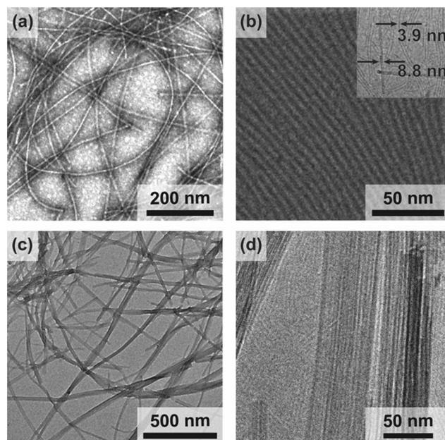
**Fig. 2** Compounds 1 and 2 self-assemble into high aspect ratio nanoribbons in water. (a) Conventional TEM of 1 illustrates its assembly into microns-long nanoribbons. (b) Cryogenic TEM of 1 reveals a  $3.9 \text{ nm} \times 8.8 \text{ nm}$  nanoribbon cross-section (inset). (c) Conventional TEM of 2 shows bundling of microns-long nanoribbons. (d) Cryogenic TEM of 2 nanoribbons identifies a  $3.9 \times 5.1 \text{ nm}$  cross-section.
