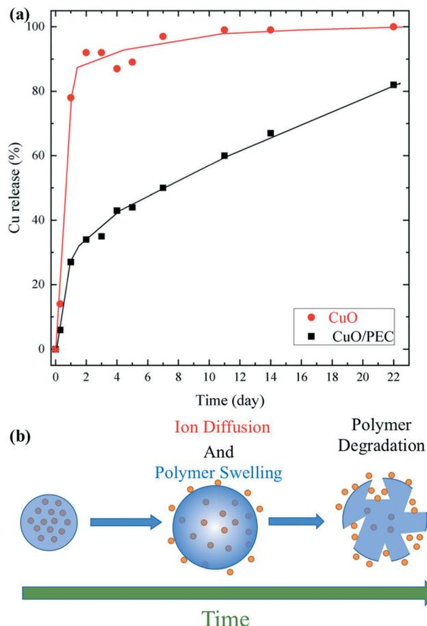
**Fig. 6** (a) Cumulative percentage release of Cu versus time from CuO nanopowder and the CuO/PEC NPs, under a constant of pH = 5.5. (b) Schematic of the mechanism of Cu release from the CuO/PEC nanocomposite.
