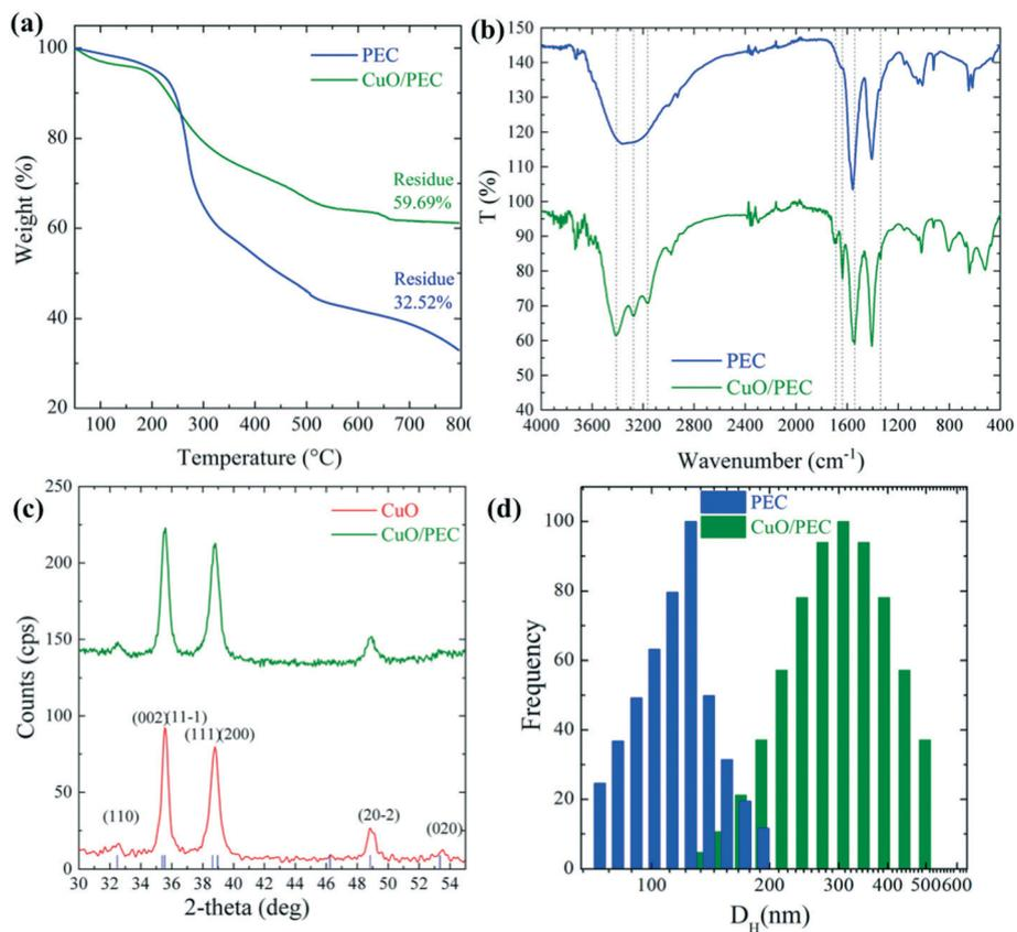
**Fig. 2** (a) Thermogravimetric profiles of the PEC (blue trace) and CuO/PEC (green trace) samples. (b) Fourier-transform infrared spectra of PEC and CuO/PEC. Dashed lines refer to peaks indicative of the CuO/PEC complex formation. (c) X-ray diffraction patterns of the CuO/PEC and CuO nanopowder. The indexed peaks for the monoclinic CuO lattice are reported [JCPDS no. 41-0254]. (d) Hydrodynamic diameter,  $D_H$ , distributions for the PEC and CuO/PEC samples.
