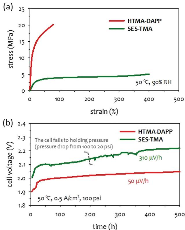
Fig. 16 (a) Stress–strain curves of HTMA-DAPP and SES-TMA AEMs. (b) Comparison of long-term performance of AEMWEs using HTMA-DAPP (78  $\mu\text{m}$  thick) and SES-TMA (53  $\mu\text{m}$  thick) AEMs. Ionomer: Aemion,  $\text{Co}_3\text{O}_4$  ( $3 \text{ mg cm}^{-2}$ ), cathode: Pt black ( $3 \text{ mg}_{\text{Pt}} \text{ cm}^{-2}$ ). The AEMWE cell data was produced at Nel Hydrogen.
