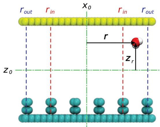
Fig. 4 Partitioning of the confinement along coordinate  $x$ . The central region between the red vertical lines corresponds to the uniform field and the outer regions between the blue and red lines feature a gradual decay of the field vanishing at the confinement boundary ( $|x| = r_{\text{out}}$ ).
