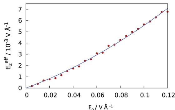
Fig. 5 Average screened electric field  $E_z^{\text{eff}}$  spanning the aqueous slab in the confinement as a function of the input (nonscreened) field  $E_0$ . The ratio  $E_0/E_z^{\text{eff}} \sim 25.5$  at  $E_z = 0$  and  $\sim 17$  at the strongest field provides an estimate for the effective dielectric constant ( $\langle 1/\epsilon_{zz} \rangle^{-1}$ ) inside the water slab at different field strengths. Reduction with the field reflects dielectric saturation.
