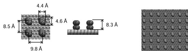
Fig. 1 Topological details (left) and top view (right) of the corrugated surface. The posts of specified dimensions are planted along lateral ( $x,y$ ) directions on the surface, which spans the entire box in the  $y$  direction, while it is of finite width smaller than the width of the box in the  $x$  direction. The system is periodically replicated along the  $x$  and  $y$  directions.
