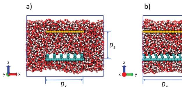
Fig. 2 Side views of field-free (the Cassie state) simulation box from the (a)  $y$  and (b)  $x$  directions. The superhydrophobic surface is shown in cyan and the weakly hydrophilic confinement wall at height  $D_z = 40 \text{ \AA}$  in yellow. The superhydrophobic area has a finite width ( $54 \text{ \AA}$ ) along the  $x$  axis. In view of lateral periodicity, the surface is of infinite length in the  $y$  direction.
