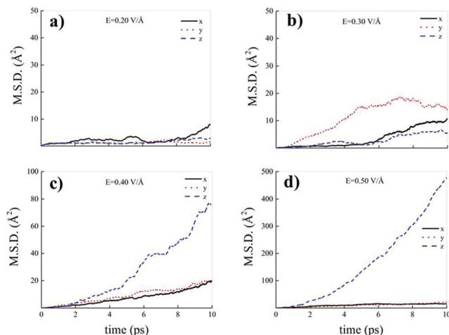
Fig. 9 Cartesian components of the mean squared displacement (MSD) of the hydrogen atoms belonging to water molecules composing the methane–water mixture at field strengths equal to  $0.20 \text{ V } \text{Å}^{-1}$  (a),  $0.30 \text{ V } \text{Å}^{-1}$  (b),  $0.40 \text{ V } \text{Å}^{-1}$  (c), and  $0.50 \text{ V } \text{Å}^{-1}$  (d).
