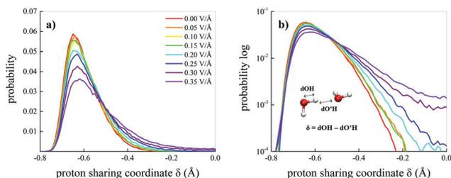
Fig. 6 Proton sharing in H-bonds. Probability distributions in the linear (a) and logarithmic (b) scale of the proton sharing coordinate  $\delta$  of water in the methane–water mixture under the effect of static electric fields at different intensities (see the legend in (a)). In the inset of (b), the definition of the coordinate, which is defined for every hydrogen atom involved in a tight H-bond (*i.e.*,  $\delta \geq -0.8$ ), is shown.
