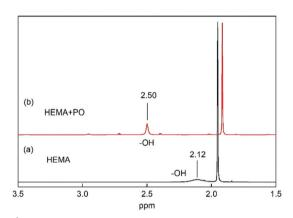
Fig. 8  $^{-1}$ H NMR spectra of HEMA with and without PO in CDCl $_3$ . (a) HEMA 10  $\mu$ L, CDCl $_3$  0.5 mL. (b) PO 30  $\mu$ L, HEMA 10  $\mu$ L, CDCl $_3$  0.5 mL.
