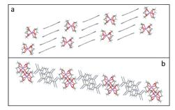
Fig. 8 Side (a) and top (b) views of the sheets of face-to-face  $\pi$ -stacked columns of TCNQ dimers formed in (12-crown-4)<sub>2</sub>Li(TCNQ)<sub>2</sub> (3), revealing the long-axis slipped character of the TCNQ dimer.
