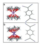
Fig. 1 Unit cell of TCNQ complexes (a). (12-crown-4)<sub>2</sub>LiTCNQ (1) and (b). (12-crown-4)2NaTCNQ (2). In each case, the 12-crown-4 ether ligands are disordered
