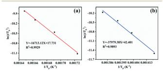
Fig. 8 Plots of  $\ln(\beta/T_{\rm p}^2)$  versus reciprocal peak temperature  $1/T_{\rm p}$  for different specimens: (a) the mixture of AP with the Cu<sub>2</sub>O hollow spheres; (b) pure AP.
