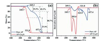
Fig. 6 (a) TG and (b) DTG curves for pure AP and the mixture of AP with the Cu<sub>2</sub>O hollow spheres.
