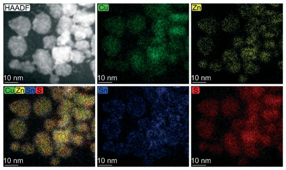
Fig. 3 Elemental map based on EDX analysis carried out on CZTS particles synthesized under solvothermal conditions at 200 °C for 2 h.
