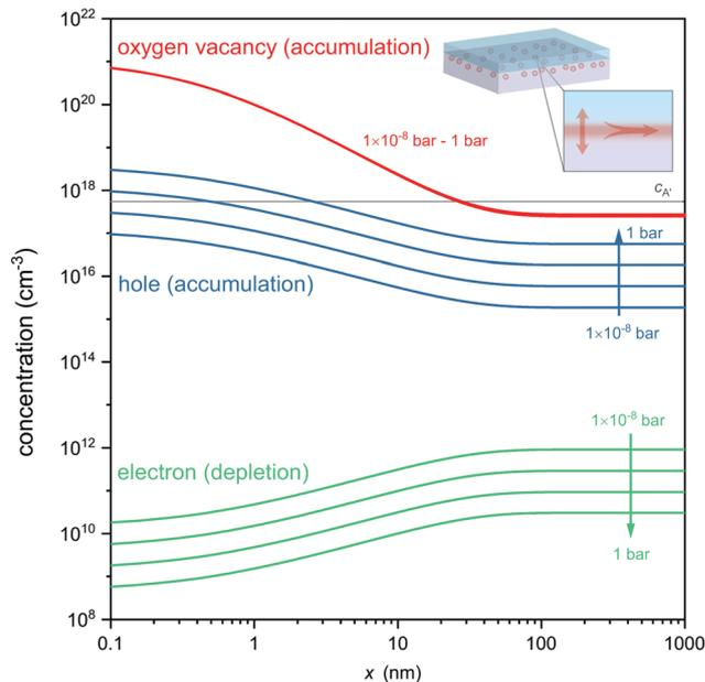
Fig. 4 Defect concentration profiles at the p-type LaAlO<sub>3</sub>/SrTiO<sub>3</sub> interface calculated for different oxygen pressures. The accumulation layer of oxygen vacancies (red lines) is robust against a variation of  $p\text{O}_2$ , and exceeds the hole concentration (blue) as well as the impurity concentration (gray line) by orders of magnitude.
