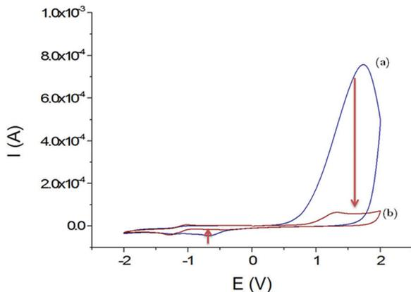
Fig. 3 Voltammograms obtained in  $\text{CH}_3\text{CN} + 0.1 \text{ mol L}^{-1}$  TBAP; first cycle (a) and second cycle (b) with the GCE/ $\text{WS}_2\text{-COOH}$  modified electrode between  $-2.0$  and  $+2.0 \text{ V}$  vs.  $\text{Ag}^+/\text{Ag}$ ; scan rate:  $100 \text{ mV s}^{-1}$ .
