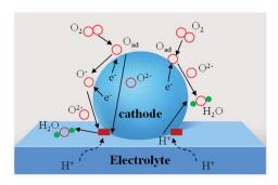
Fig. 1 Schematic diagram of R-P cathode with different transportation routes (including  $e^-$ ,  $O^{2-}$ ,  $H^+$ ).
