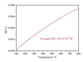
Fig. 7 The thermal expansion coefficient of PrBaNiMn over the temperature range of 100–800  $^{\circ}\text{C}.$
