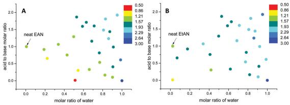
Fig. 12 The change in Gordon parameters of (A) EAN derived and (B) EtAN derived solvent compositions in J mol<sup>1/3</sup> m<sup>-3</sup>.
