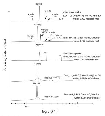
**Fig. 4** SAXS patterns of 70 wt% CTAB in base-rich EAN compositions at 65 °C. The symbol  $L_c$ -1 denotes a lamellar surfactant crystalline phase, and the liquid crystal phases are denoted as normal hexagonal ( $H_1$ ) and normal primitive cubic ( $V_1$  ( $Im\bar{3}m$ )) liquid crystal phases.
