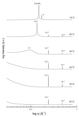
Fig. 2 SAXS patterns of 70 wt% CTAB in neat EtAN at temperatures between 25 to 75 °C. The liquid crystal phases are denoted as micellar  $(L_1)$ , normal hexagonal  $(H_1)$ , and unassigned transient (U) liquid crystal phases. The symbols  $L_c$ -1 and  $L_c$ -4 denote lamellar surfactant crystalline phases
