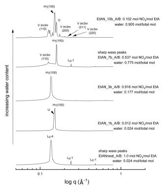
**Fig. 5** SAXS patterns of 70 wt% CTAB in base-rich EtAN compositions at 65 °C. The symbols  $L_c$ -1 and  $L_c$ -4 denote lamellar surfactant crystalline phases, and the liquid crystal phases are denoted as normal hexagonal ( $H_1$ ), normal primitive cubic ( $V_1$  ( $Im\bar{3}m$ )), lamellar ( $L_{\alpha}$ ), and unassigned transient (U) liquid crystal phases.
