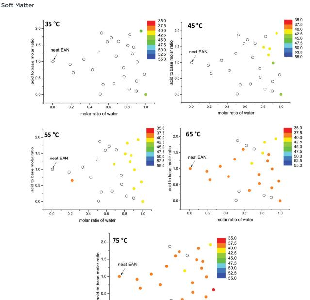
Fig. 10 The change in lattice parameter values (Å) of the hexagonal phase ( $H_1$ ) of 70 wt% CTAB in EAN derived solvent compositions as a function of temperature. Solid data points represent the sample compositions when the phase formation is supported while blank data points only denote sample compositions with this phase not observed.
