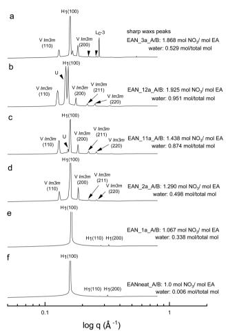
Fig. 6 SAXS patterns of 70 wt% CTAB in acid-rich EAN compositions at 65 °C. The symbol L<sub>c</sub>-3 denotes a lamellar surfactant crystalline phase, and the liquid crystal phases are denoted as normal hexagonal (H<sub>1</sub>), normal primitive cubic ( $V_1$  ( $Im\bar{3}m$ )), and unassigned transient (U) liquid crystal phases
