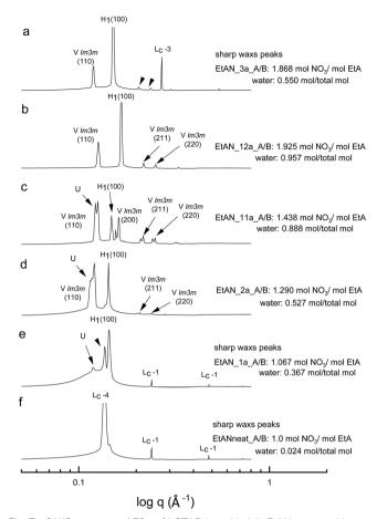
SAXS patterns of 70 wt% CTAB in acid-rich EtAN compositions at 65 °C. The symbols L<sub>c</sub>-1 to L<sub>c</sub>-4 denote lamellar surfactant crystalline phases, and the liquid crystal phases are denoted as normal hexagonal (H<sub>1</sub>), normal primitive cubic ( $V_1$  ( $Im\bar{3}m$ )), and unassigned transient (U) liquid crystal phases, respectively.
