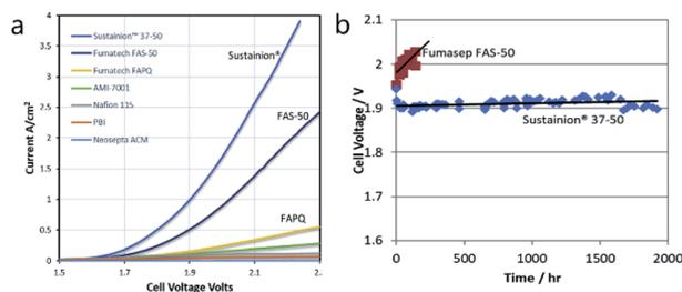
**Fig. 9** (a) Comparison of current–voltage response of AEM electrolysis with various membranes in ref. 119. (b) Steady state voltage performance at  $1 \text{ A cm}^{-2}$  with Sustainion 37–50 membrane and FAS-50 membrane ( $60 \text{ }^\circ\text{C}$ ,  $1 \text{ M KOH}$ ,  $\text{NiFe}_2\text{O}_4$  anode and  $\text{NiFeCo}$  cathode). Reprinted from ref. 125 with permission from Elsevier.<sup>125</sup>
