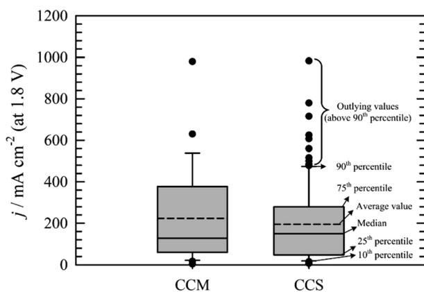
Fig. 6 Comparison of the current densities achieved at cell voltage  $1.8 \text{ V}$  using the CCM<sup>57,59,106,107,114,116,131–136,139–141</sup> or CCS<sup>22,54,55,95,101–104,108,109,111–113,115,117–124,126–129,142,143</sup> method of MEA construction.
