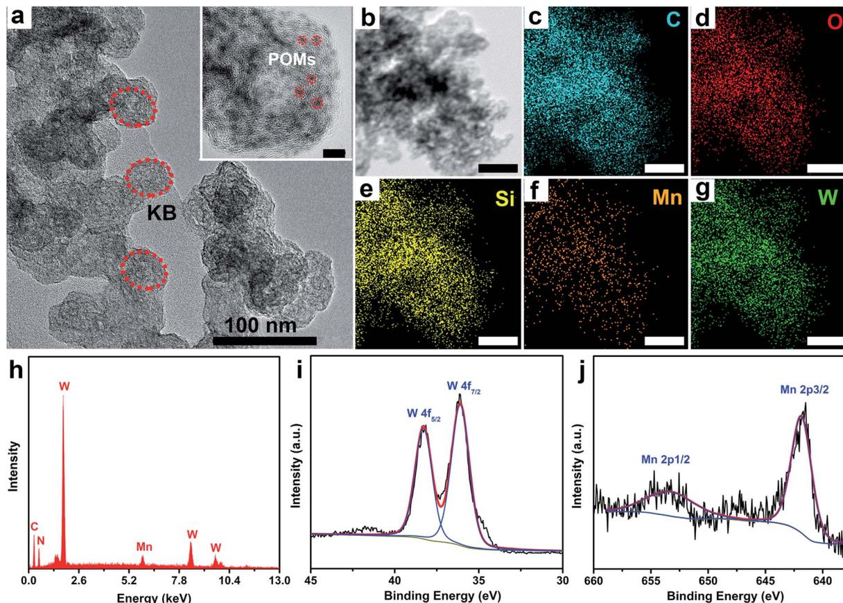
Fig. 1 (a) TEM images of SiW<sub>12</sub>-MnL/KB (inset: HR-TEM images of SiW<sub>12</sub>-MnL/KB, scale bar: 5 nm). (b–g) Corresponding elemental mapping of C, O, Si, Mn and W of SiW<sub>12</sub>-MnL/KB, scale bar: 100 nm. (h) The EDX spectra of SiW<sub>12</sub>-MnL/KB. (i and j) The XPS spectra of SiW<sub>12</sub>-MnL/KB: (i) W, (j) Mn.
