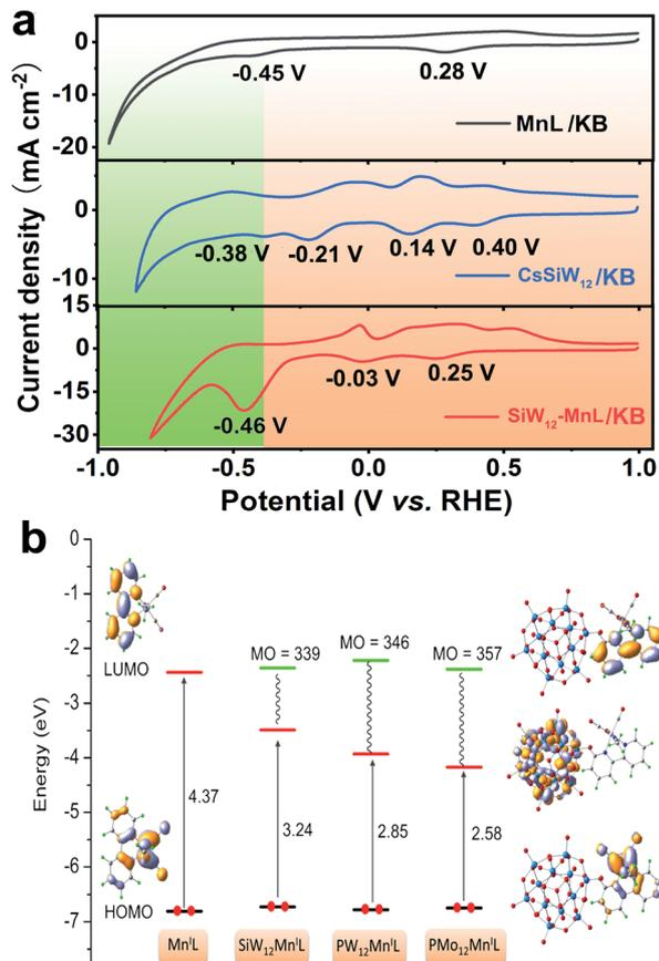
Fig. 2 (a) The CVs for MnL/KB, CsSiW<sub>12</sub>/KB and SiW<sub>12</sub>-MnL/KB in 0.5 mol L<sup>-1</sup> N<sub>2</sub>-saturated KHCO<sub>3</sub> at a 0.05 V s<sup>-1</sup> scan rate. (b) Computed frontier orbitals (compositions and energies) for MnL, SiW<sub>12</sub>-MnL, PW<sub>12</sub>-MnL, and PMO<sub>12</sub>-MnL (the green lines represent the unoccupied molecular orbitals (MO) contributed by MnL in POM-MnL).
