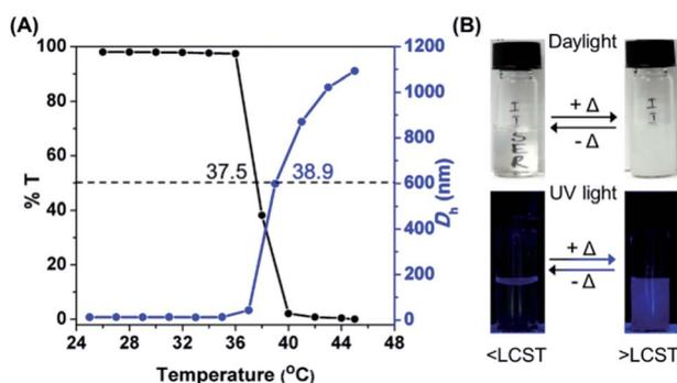
Fig. 3 (A) Variation of %T and  $D_h$  of a 0.1 wt% aqueous PNVCL solution as a function of temperature. (B) Photographs of the same PNVCL solution acquired under daylight and UV irradiation (365 nm) below and above the LCST.
