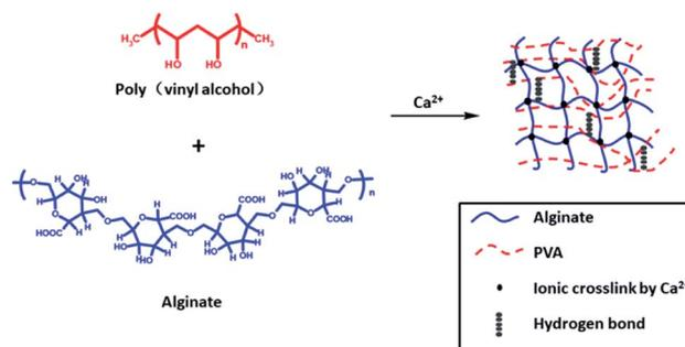
Fig. 2 Physically cross-linked sodium alginate-based semi-IPN hydrogel film formation mechanism. This figure has been adapted from ref. 52 with permission from John Wiley & Sons, Ltd., Copyright © 2008.
