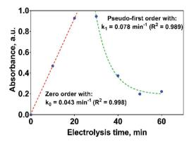
Fig. 10 Kinetic parameters for the formation and consumption of 2,4-DP as first reaction intermediate on the Si/BDD anode in  $0.5 \text{ M Na}_2\text{SO}_4$  + 100 ppm 2,4-DNa solution at 30 mA cm<sup>-2</sup> and 298 K.
