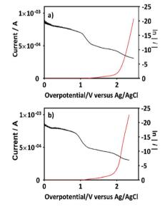
Fig. 13 The variation of current as a function of the overpotential ( $\eta$ ) for BDD in (a) 0.5 M NaClO<sub>4</sub> solution and (b) 0.5 M NaClO<sub>4</sub> + 100 ppm 2,4-DNa (pH 3) solution at 10 mV s<sup>-1</sup> and 298 K. The Tafel analysis is included for each one case in the corresponding figure (plotting ln(i) against  $\eta$ ).
