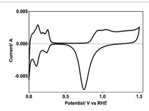
Fig. 1 Voltammogram of the Pt electrode used as cathode, recorded in 0.5 M H<sub>2</sub>SO<sub>4</sub> as supporting electrolyte at v = 50 mV s<sup>-1</sup> and at 298 K.
