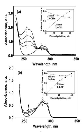
Fig. 14 UV spectra for  $100~\rm mg~L^{-1}$  2,4-DNa solutions in  $0.5~\rm M~Na_2SO_4$  electrolyzed at  $30~\rm mA~cm^{-2}$  and  $298~\rm K$ , as a function of the electrolysis time and on (a) Pb/PbO<sub>2</sub> and (b) Ti/Sb-doped SnO<sub>2</sub> anodes, respectively. The corresponding insets show the variation of the relative absorbance for both 258 and 285 nm UV bands.
