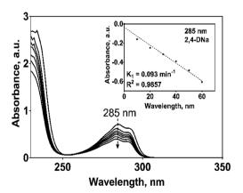
Fig. 12 UV spectra, as a function of the electrolysis time, for 100 mg  $\rm L^{-1}$  2,4-DNa solutions in 0.5 M NaClO $_4$  electrolyzed on a Si/BDD anode at 30 mA cm $^{-2}$  and 298 K. Inset shows the pseudo-first order graphic of the UV band decrease at 285 nm.
