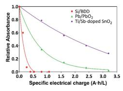
Fig. 6 Plots of the relative absorbance of MR again specific electrical charge (A h L<sup>-1</sup>) for solutions containing 20 mg L<sup>-1</sup> MR in 0.5 M H<sub>2</sub>SO<sub>4</sub> at 30 mA cm<sup>-2</sup> and 298 K:  $\bullet$  Si/BDD,  $\bullet$  Ti/Sb-doped SnO<sub>2</sub>,  $\blacktriangle$  Pb/PbO<sub>2</sub>.
