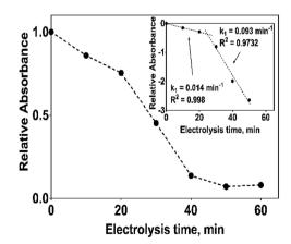
Fig. 9 Plot of the relative absorbance at 285 nm of 2,4-DNa as a function of the electrolysis time for the electrolysis of a solution containing 100 mg  $L^{-1}$  2,4-DNa in 0.5 M  $\rm Na_2SO_4$  at 30 mA cm $^{-2}$  and 298 K on Si/BDD anode. Inset shows the corresponding pseudo-first order graphic.
