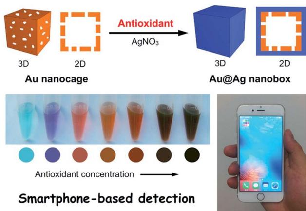
Fig. 3 The sensing principle of antioxidant based on the morphological change of Au nanocage upon the reduction of  $\text{AgNO}_3$  producing Au@Ag nanobox in presence of antioxidants. Adapted from ref. 48 with permission from Royal Society of Chemistry, Copyright 2018.
