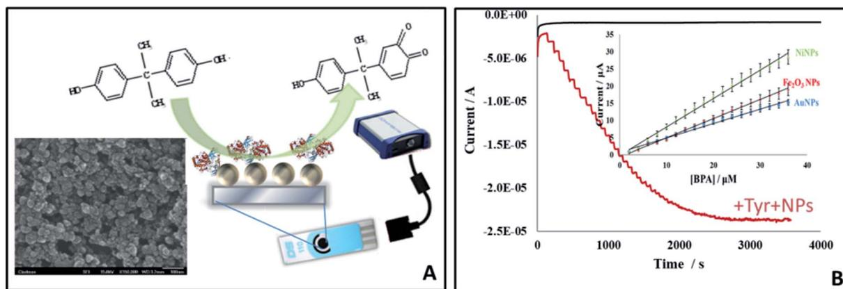
Fig. 5 Enzyme-based detection of BPA by NP amplification using screen printed electrodes modified with Au, Ni or  $\text{Fe}_2\text{O}_3$  NPs: sensor design (A) and amperometric response with comparative calibration curve (B) showing differential responses to the three types of NPs of which Ni NPs showed the highest sensitivity (schematic summarizing detection platform and results reported in ref. 33).
