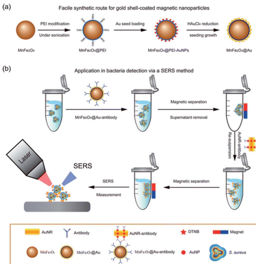
Fig. 9 (a) Synthesis of MnFe<sub>2</sub>O<sub>4</sub>@Au core/shell NPs and (b) SERS method of *Staphylococcus aureus* detection. Adapted with permission from (ref. 32, Copyright (2016) American Chemical Society).
