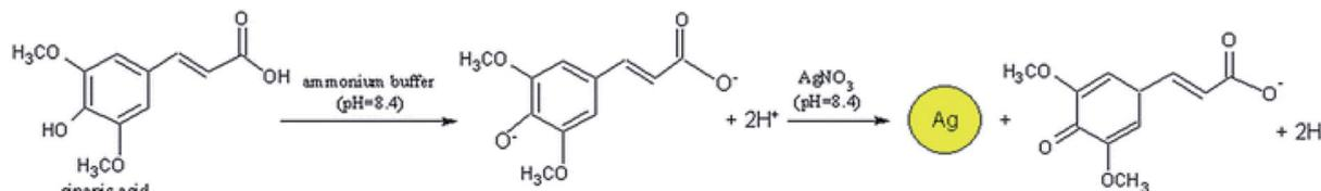
Fig. 2 The oxidation of  $\text{Ag}^+$  with the antioxidant sinapic acid resulted in production of AgNPs which can be detected spectrophotometrically. Adapted from ref. 47 with permission from Royal Society of Chemistry, Copyright 2012.
