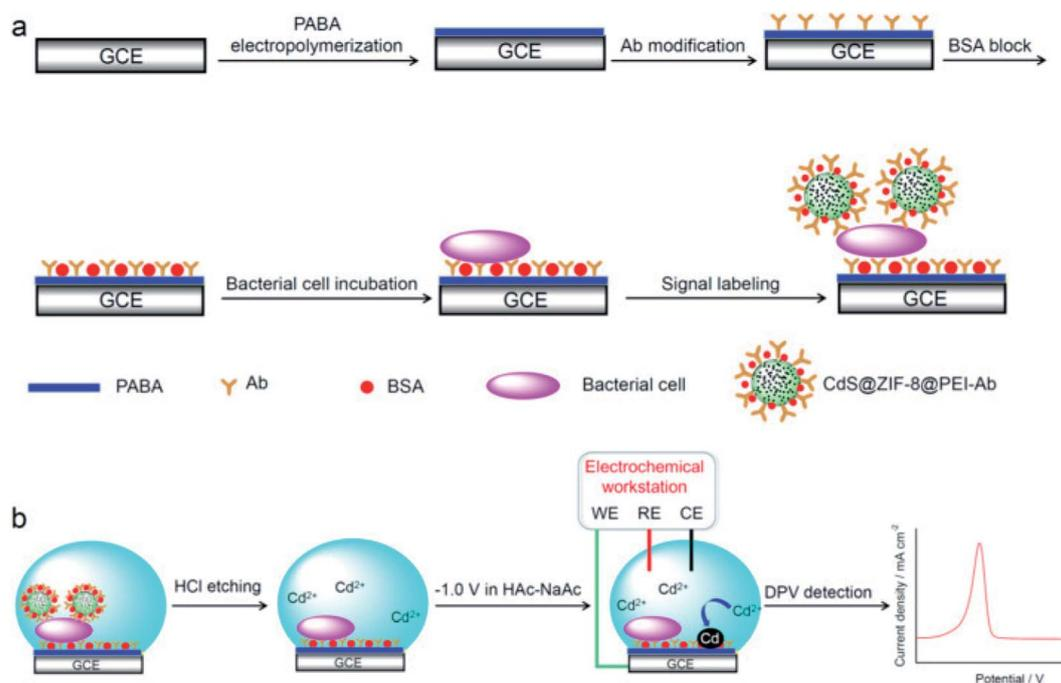
Fig. 8 (a) Fabrication of sandwiched electrochemical immunosensor for detection of *E. coli*: GCE was modified with poly(*p*-aminobenzoic acid) (PABA) followed by anti-*E. coli* O157:H7 Ab covalent immobilization, blocking with bovine serum albumin (BSA), *E. coli* incubation and finally labelling with CdS@ZIF-8@PEI-Ab tags. (b) Electrochemical detection of leached Cd(II) resulting from etching of CdS@ZIF-8@PEI-Ab tag. Adapted from ref. 78 with permission from Elsevier B.V., Copyright 2018.
