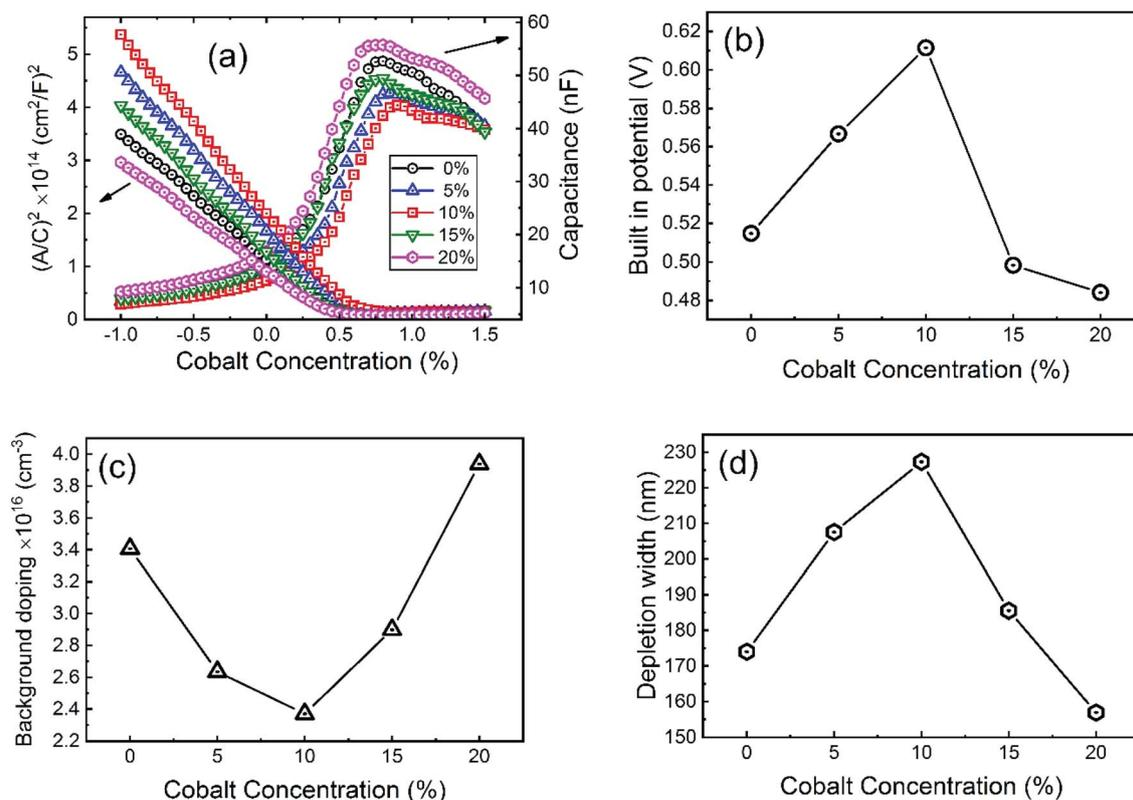
Fig. 14 (a) Capacitance–voltage ( $C$ - $V$ ) and Mott–Schottky plots of the 0–20% cobalt doped  $\text{ZnO}/\text{CuO}$  heterojunction solar cells. Variation in (b) built-in potential, (c) background doping concentration, and (d) depletion width as a function of cobalt concentration.
