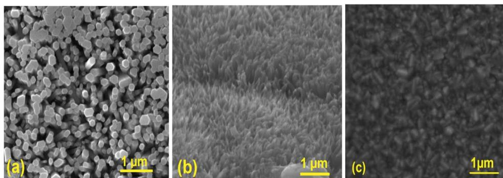
Fig. 3 SEM images of (a) undoped ZnO nanorods (b) CuO nanostructures (c) MoO<sub>3</sub> thin film.
