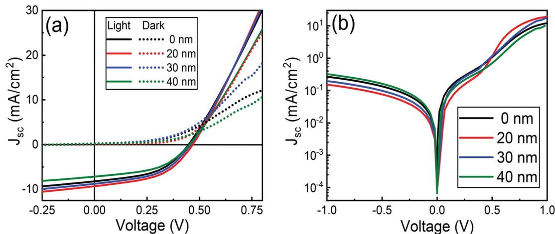
Fig. 15 (a)  $I$ - $V$  characteristics under light and dark of 10% cobalt doped ZnO/CuO/MoO<sub>3</sub> heterojunction solar cells with a different thickness of the MoO<sub>3</sub> buffer layer. (b) Semi-log plot of dark  $I$ / $V$  for one diode model fit.
