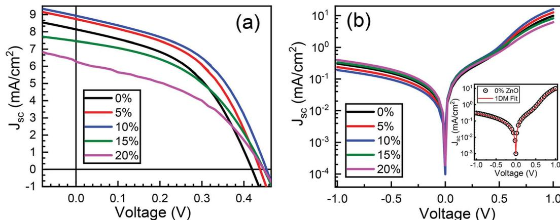
Fig. 9 (a)  $I$ - $V$  characteristics under light and (b) dark  $I$ - $V$  characteristics of 0–20% cobalt doped ZnO/CuO heterojunction solar cells. The insets of (b) show one diode model fit of 0% ZnO/CuO solar cell.
