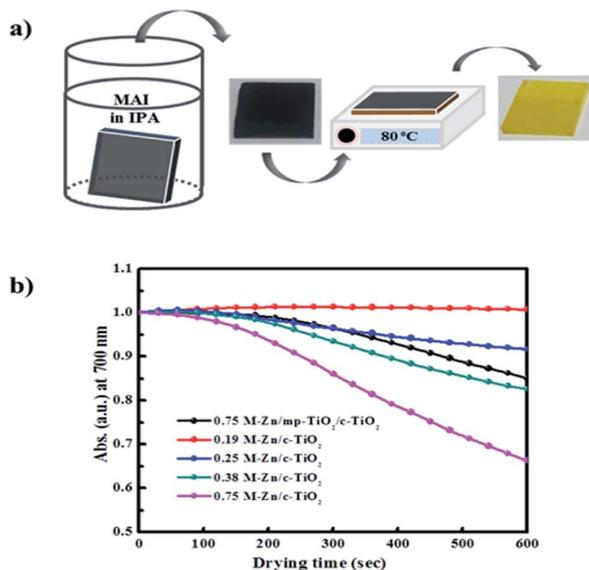
Fig. 3 (a) The decomposition behaviors and (b) the decrease in the absorbance at 700 nm over 600 s of the MAPbI<sub>3</sub> perovskite film fabricated by this sequential dip-coating deposition on ZnO/c-TiO<sub>2</sub> layer observed during solvent drying.
