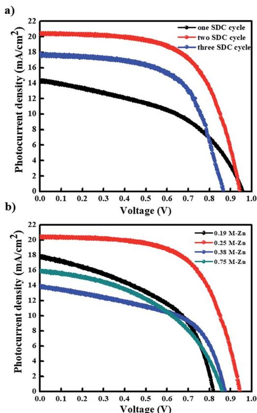
Fig. 7 Current–voltage (*J*–*V*) curves under AM 1.5 irradiation (100 mW cm<sup>-1</sup>) for the PHJ PrSCs based on (a) MAPbI<sub>3</sub> perovskite layers fabricated by the designated number of SDC cycles followed by three SSIER cycles on ZnO (0.25 M-Zn) over the c-TiO<sub>2</sub> layers, and (b) MAPbI<sub>3</sub> perovskite layers fabricated on ZnO (0.19 M-Zn), ZnO (0.25 M-Zn), ZnO (0.38 M-Zn), and ZnO (0.75 M-Zn) over the c-TiO<sub>2</sub> layers under two SDC cycles.
