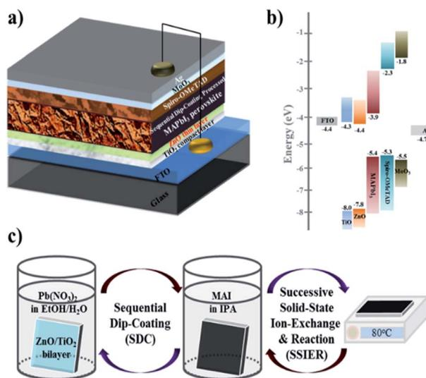
Fig. 1 Description of (a) PHJ PrSC structure, (b) energy level diagram, and (c) the preparation of the MAPbI<sub>3</sub> perovskite films by sequentially dip-coating a ZnO-covered c-TiO<sub>2</sub>/FTO substrate in aqueous Pb(NO<sub>3</sub>)<sub>2</sub> and MAI solutions.
