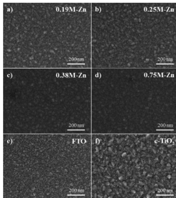
Fig. 2 SEM surface topologies of thin ZnO layers fabricated from ZnO sol-gel precursors prepared with various Zn concentrations of (a) 0.19 M-Zn, (b) 0.25 M-Zn, (c) 0.38 M-Zn, and (d) 0.75 M-Zn over the c- $\text{TiO}_2$  layer, which were compared to those of the (e) bare FTO substrate and (f) c- $\text{TiO}_2$  layer deposited on the FTO.
