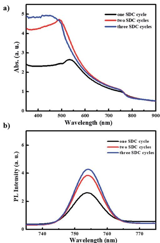
Fig. 5 (a) UV-vis absorption and (b) photoluminescence spectra for these PHJ  $\text{MAPbI}_3$  perovskite films deposited on  $\text{ZnO}$  (0.25 M-Zn)/ $\text{c-TiO}_2/\text{FTO}$  under designed SDC cycles.
