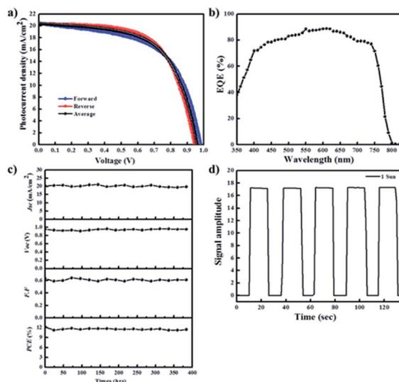
Fig. 8 (a) The hysteresis of the *J*–*V* curves in both scan directions under AM 1.5 irradiation (100 mW cm<sup>-1</sup>), (b) EQE spectra, (c) stability, and (d) photoswitching phenomenon for the most efficient PHJ PrSCs fabricated using dip-coating deposition approach on the thin ZnO/c-TiO<sub>2</sub> bilayer ETL under two SDC cycles.
