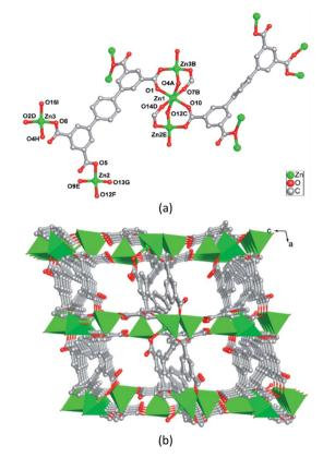
Fig. 1 (a) Representation of the Zn(II) coordination environments in 1. Symmetry codes (A) 1+X, +Y, +Z; (B) 1+X, 1+Y, +Z; (C) -1+X, -1+Y, +Z; (E) -X, 1-Y, -Z; (F) 1-X, 1-Y, -Z; (G) 1-X, 2-Y, -Z; (H) +X, -1+Y, +Z; (I) 1-X, 2-Y, 1-Z. (b) View of 3D coordination framework of 1.
