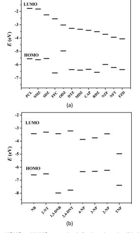
Fig. 4 HOMO and LUMO energy levels for the selected antibiotics (a) and nitroaromatics explosives (b).
