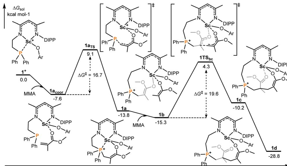
Fig. 1 Computed energy profiles (M06(SMD)/6-311G\*\*nSDD//B3PW91/6-31G\*\*nSDD), see the ESI† for more details for  $1^+$  mediated polymerization of MMA (intramolecular RE/P systems). Free energies ( $\text{kcal mol}^{-1}$ ) are relative to isolated reactants.
