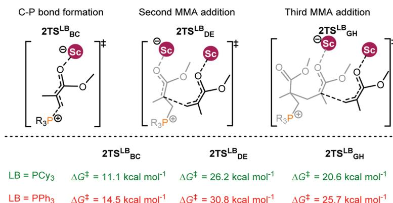
Fig. 6 Transition states for MMA polymerization initiated by the  $2/\text{R}_3\text{P}$  pair ( $\text{R} = \text{Cy}$  and  $\text{Ph}$ ). Free energies ( $\text{kcal mol}^{-1}$ ) are relative to isolated reactants.
