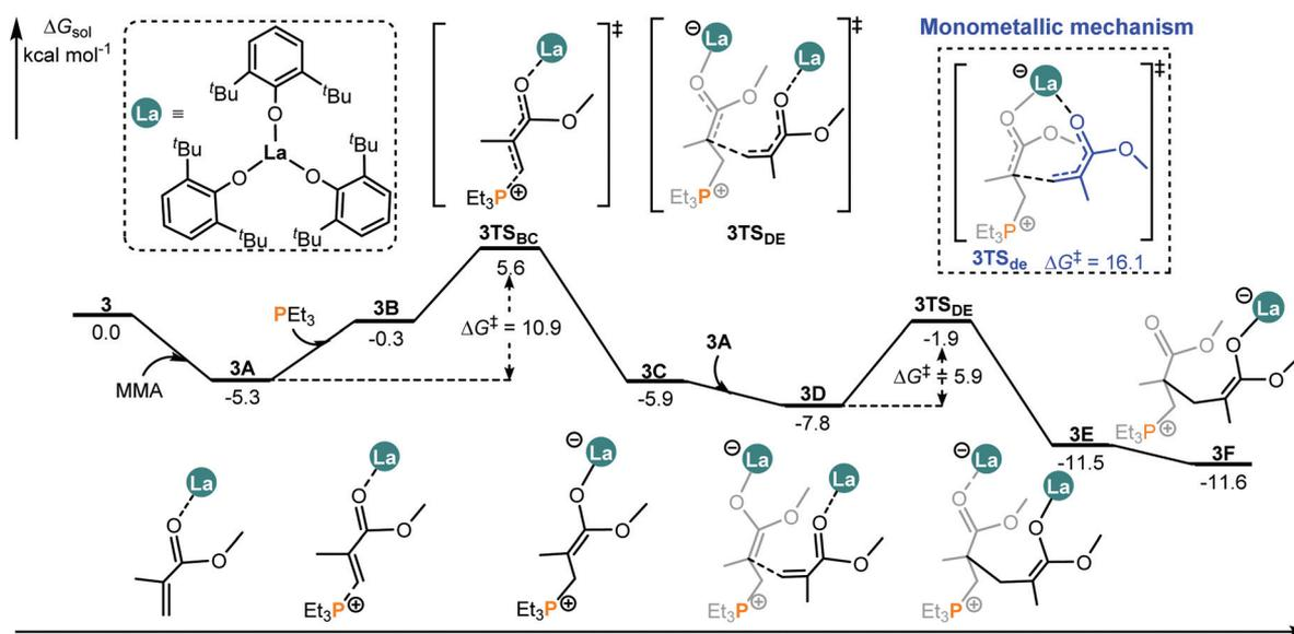
Fig. 4 Computed energy profiles for the 3/ $\text{PEt}_3$  mediated (intermolecular RE/P systems) bimetallic pathway for MMA enchainment. Free energies ( $\text{kcal mol}^{-1}$ ) are relative to isolated reactants.
