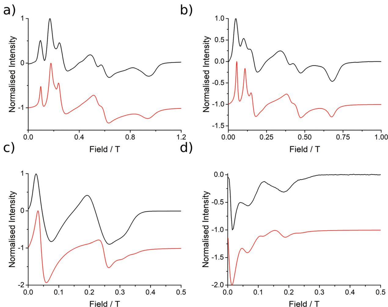
**Fig. 3** EPR spectra (black lines) collected at 5 K for **1** at (a) Q-band (33.970818 GHz), (b) K-band (23.791 GHz), (c) X-band (9.37198 GHz) and (d) S-band (3.87285 GHz), with simulations in red from the parameters presented in Table 1.
