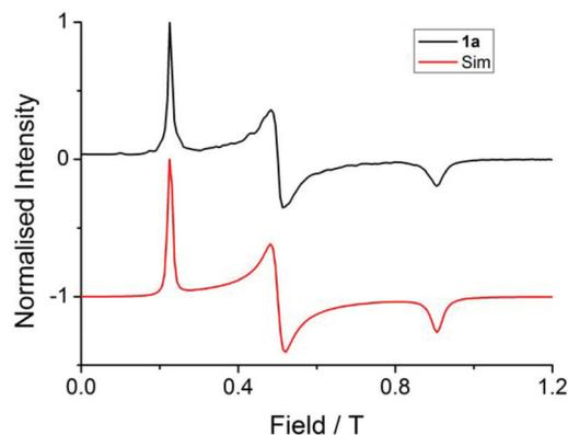
Fig. 2 Q-Band EPR measurement at 33.995818 GHz collected at 5 K on the 5% diluted **1a** [Y{5%Er}<sub>2</sub>(HMeQ\*)<sub>2</sub>(NO<sub>3</sub>)<sub>6</sub>] (black) with the fitted spectrum (red), following the procedure outlined in previous work.<sup>27</sup> *g*-Values are in Table 1, linewidths: *lw*<sub>1</sub> = 1.7, *lw*<sub>2</sub> = 2.3 and *lw*<sub>3</sub> = 1.3 GHz.
