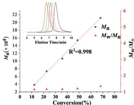
Fig. 2 Linear growth of molecular weight ( $M_n$ ) as a function of *p*F<sub>2</sub> conversion. Inset: GPC traces as detected from the retention time.
