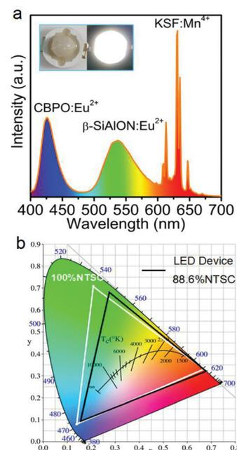
**Fig. 5** (a) Emission spectrum of w-LED fabricated by mixing blue  $\text{Ca}_2\text{Be}_2(\text{PO}_4)_2:\text{Eu}^{2+}$ , green  $\beta\text{-Sialon}:\text{Eu}^{2+}$ , and red  $\text{K}_2\text{SiF}_6:\text{Mn}^{4+}$  on a near-UV LED chip (380 nm), under 30 mA driving current. The inset shows photographs of the w-LED device taken under daylight and when it is in operation. (b) Color gamut of the NTSC standard (white triangle) and the as-fabricated w-LED device (black triangle).
