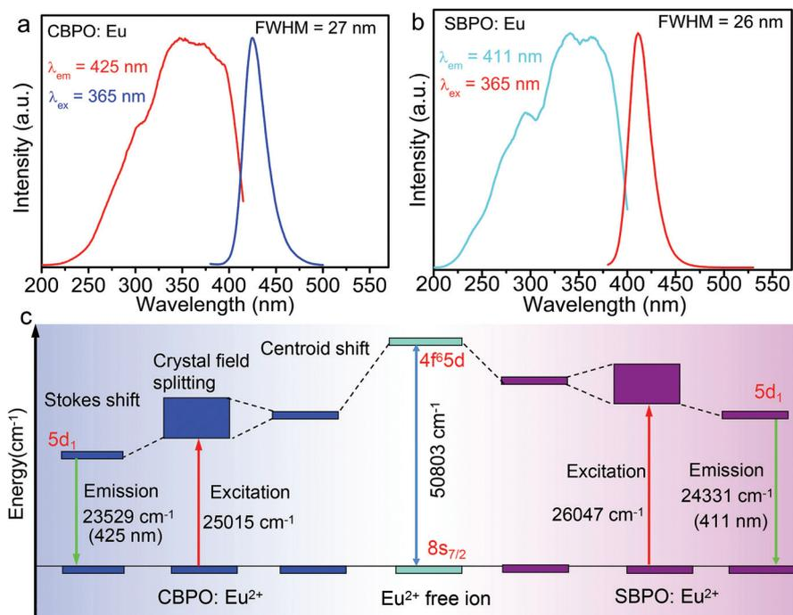
Fig. 3 Room temperature excitation and emission spectra of (a)  $Ca_2Be_2(PO_4)_2:Eu^{2+}$  and (b)  $Sr_2Be_2(PO_4)_2:Eu^{2+}$  phosphors. (c) Schematic energy level diagram for  $Eu^{2+}$  ion in  $Ca_2Be_2(PO_4)_2$  and  $Sr_2Be_2(PO_4)_2$  crystal structures.
