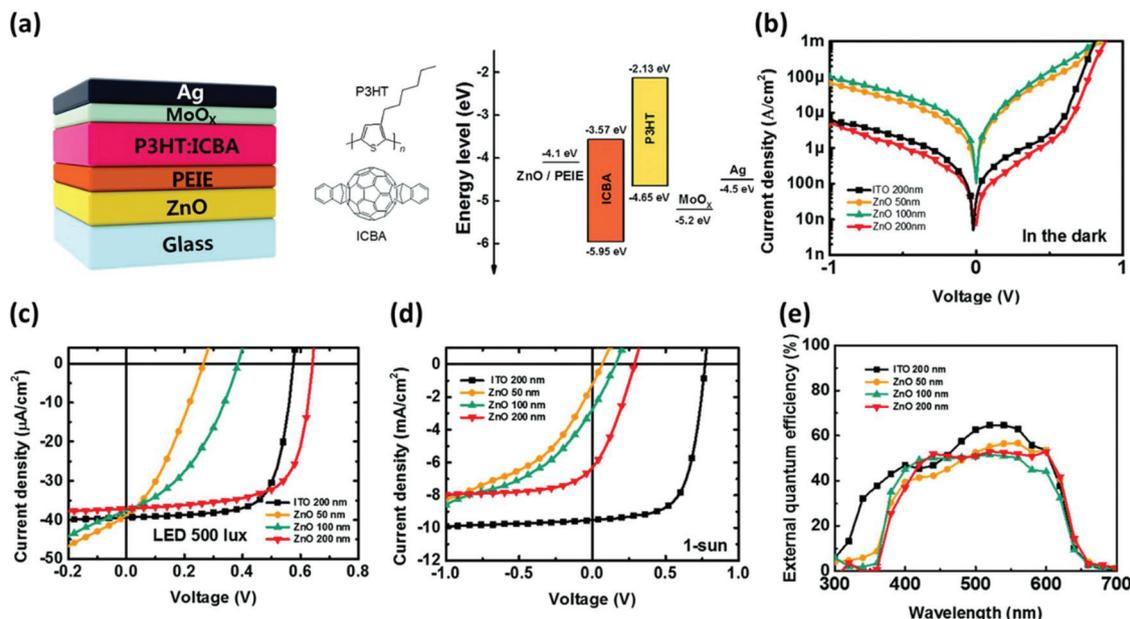
Fig. 7 Anode-free OPV devices. (a) Device structure of anode-free OPVs and the corresponding energy band diagram.  $J$ - $V$  characteristics with ITO and ZnO electrodes (with different thicknesses of 50, 100 and 200 nm) under (b) darkness, (c) 500 lx LED and (d) AM 1.5G illumination. (e) Corresponding EQE spectra. Reproduced from ref. 54 with permission from The Royal Society of Chemistry.
