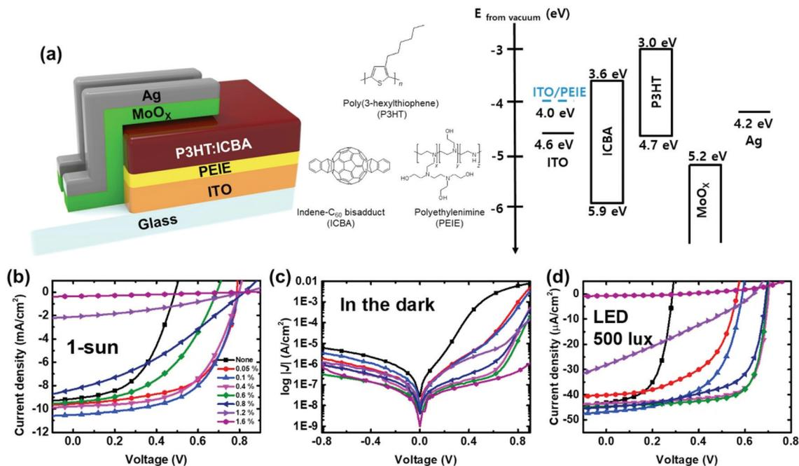
Fig. 6 PEIE thickness effect under LED illumination. (a) Device architecture, molecular structures of P3HT, ICBA and PEIE, and corresponding energy band diagram.  $J$ - $V$  characteristics measured under (b) AM 1.5G illumination, (c) darkness and (d) LED (500 lx) illumination. Reproduced from ref. 52 with permission from Elsevier.
