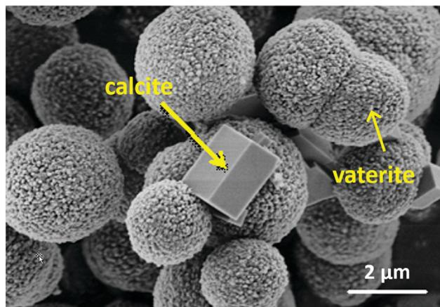
Fig. 5 SEM image of CaCO<sub>3</sub> crystals demonstrating the mesoporous nature of spherical vaterite and non-porous calcite crystals. Adopted from ref. 77, copyright© 2019, Elsevier.
