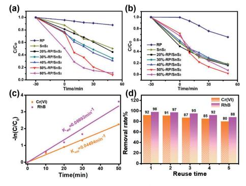
Fig. 2 Comparison of the effect of photocatalytic simultaneous removal of (a)  $Cr(v_1)$  and (b) RhB by RP, SnS<sub>2</sub>, and x-RP/SnS<sub>2</sub>, (c) the fitted reaction kinetic curves ( $-\ln(C/C_o) = kt$ ) and (d) recycling test runs for five times in the photocatalytic removal of  $Cr(v_1)$  and RhB by 50%-RP/SnS<sub>2</sub>.
