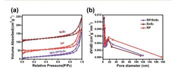
Fig. 4 (a) N<sub>2</sub> adsorption-desorption isotherms and (b) the pore size distribution of SnS<sub>2</sub>, RP and 50%-RP/SnS<sub>2</sub> samples.
