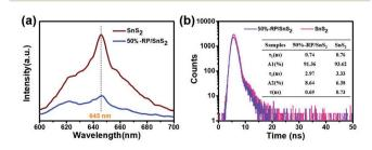
Fig. 6 (a) PL and (b) time-resolved fluorescence decay spectra and calculated average lifetime (inset) of samples.
