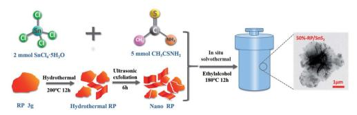
Scheme 1 Schematic illustration of the preparation of RP/SnS<sub>2</sub>
