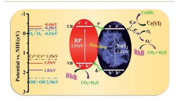
Scheme 2 Schematic illustration of photocatalytic removal mechanism of  $Cr(v_1)$  and organic pollutants over  $RP/SnS_2$  composite.
