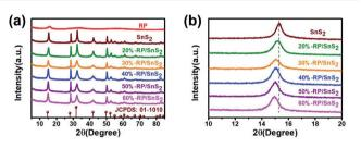
Fig. 1 XRD patterns of (a) full spectra and (b) magnified spectra of samples RP, SnS<sub>2</sub>, and x-RP/SnS<sub>2</sub>.
